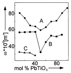
Fig. 5. The dependencies of the mode frequencies of the PZT systems on the PbTiO<sub>3</sub> concentration obtained by the Raman spectroscopy (argon laser).
