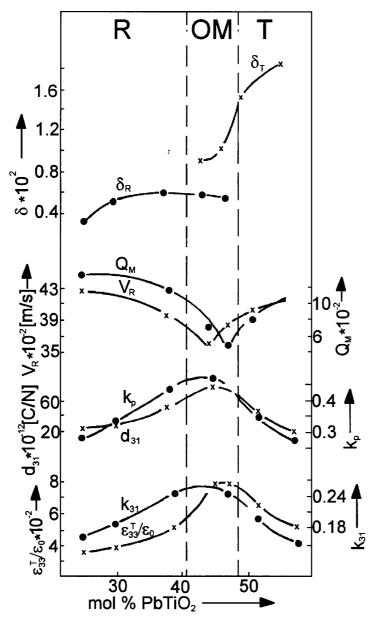
Fig. 1. The dependencies of physical parameters of the PZT-type system in the vicinity of the morphotropic phase boundary on the PbTiO<sub>3</sub> content.
