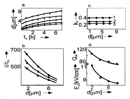
Fig. 3. The dependencies of the grain size on the sintering temperature and time (a), the dependencies of  $\varepsilon/\varepsilon_0$ , the electromechanical coupling  $(k_p)$ , coercive fields  $(E_c)$ , and mechanical quality factors  $(Q_m)$  on the grain sizes of the ceramics (b, c, d).
