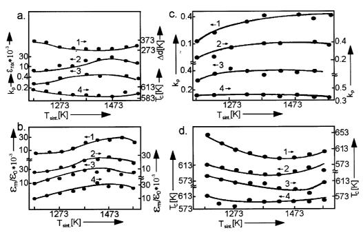
Fig. 2. The dependencies of the dielectric permittivities  $(\varepsilon_{\max})$ , electromechanical coupling coefficients  $(k_p)$ , Curie temperature  $(T_c)$  and phase transition diffuseness parameters  $(\Delta_d)$  on the sintering temperature  $(T_{sint})$  (sintering time,  $t_{sint} = 2$  hours); a) the dependencies of  $\varepsilon_{\max}$ ,  $\varepsilon_0$ ,  $k_p$ ,  $T_c$  on the sintering temperature and time  $(t_{sint}: 1-0.25; 2-2; 3-3; 4-5$  hours) (b, c, d).
