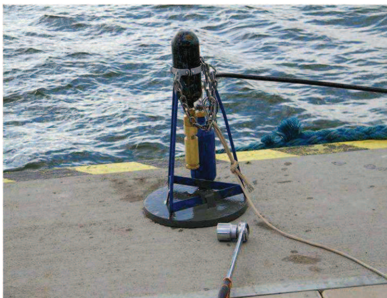
Fig. 5. Air gun model with a spring and a battery.
