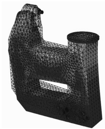
Fig. 8. C-frame deformation after maximum forming force load (clinchng joint) and its model under load condition (zoom in factor of 50).
