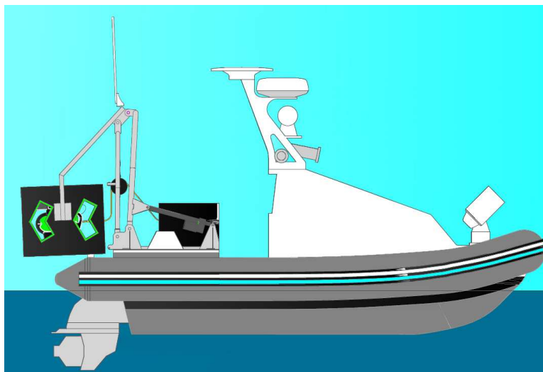
Fig. 9. Visualization of "Ededron" vehicle with an installed launch system.
