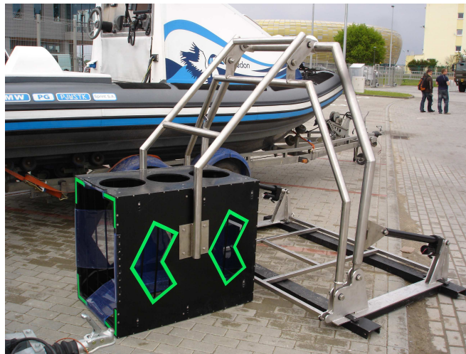
Fig. 7. Frame set of the ROV launch system with an underwater garage ready to be installed on the deck of a USV.
