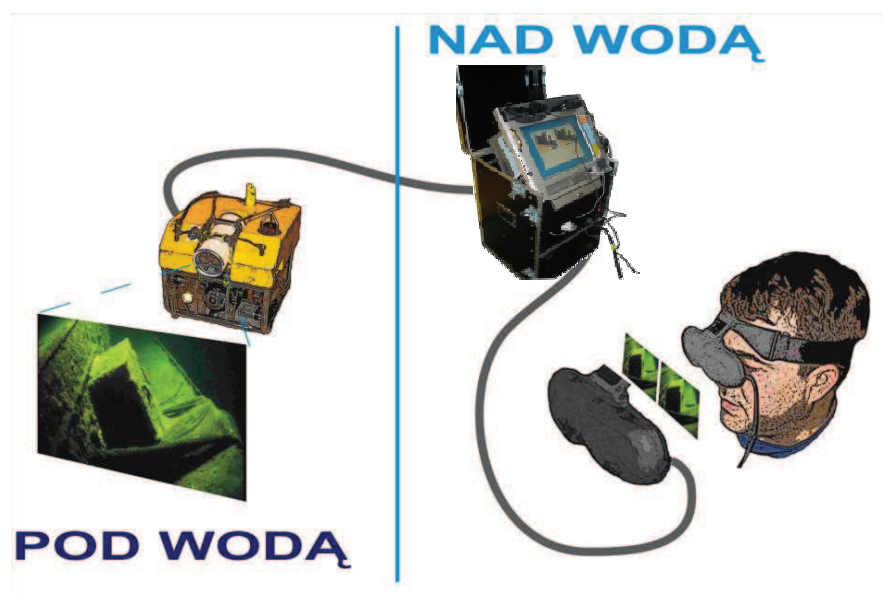
Fig. 5. A real time spacial observation system of underwater objects – ARGOOS.
