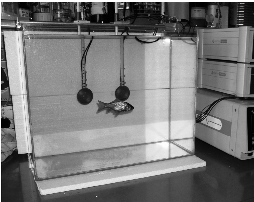
Fig. 1.2. Measuring system. Electrodes in a coplanar system (placed on one plane).
