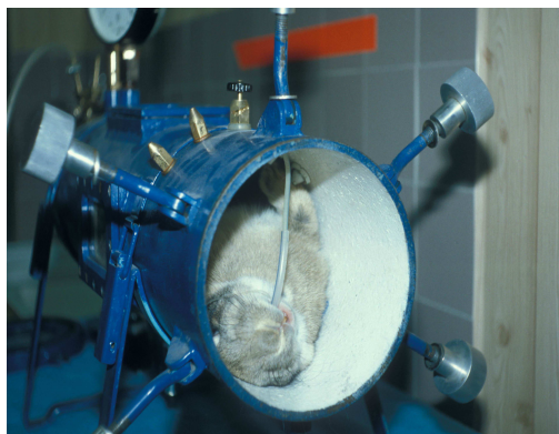
Fig. 2. Animal placement in the chamber. Visible connection of the intubation tube to the break valve.
