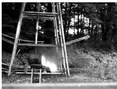
Figure 2. Photo of the ballistic mortar during firing.
