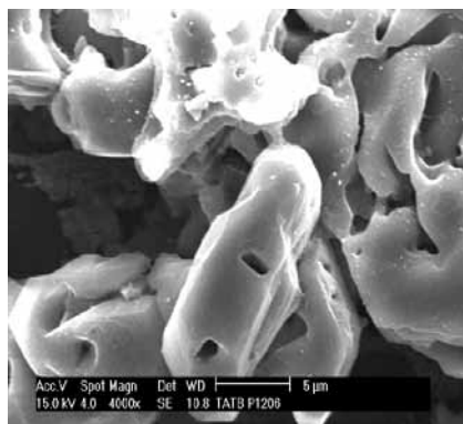
Figure 2. SEM of virgin TATB crystals.
