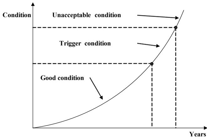
Fig. 1. The deterioration process
