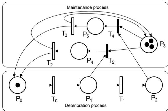
Fig. 5. The SPN of deterioration and maintenance process
