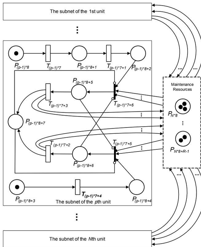
Fig. 7 The SPN of a system with N units
