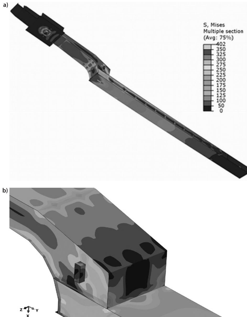
Fig. 6. H-M-H stress distribution in the modified model of the frame: a) general view b) detail of the front part of the frame
