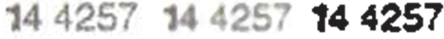
Fig. 3. Images of the digits: from the preprocessing stage, after filtration and after binarization
