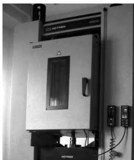
Figure 3. Instron 4500—universal tensile testing machine with a thermal chamber.
