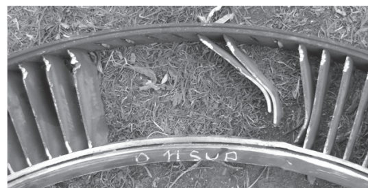
Fig. 4. Compressor stationary vane (diaphragms) damage stage 11
