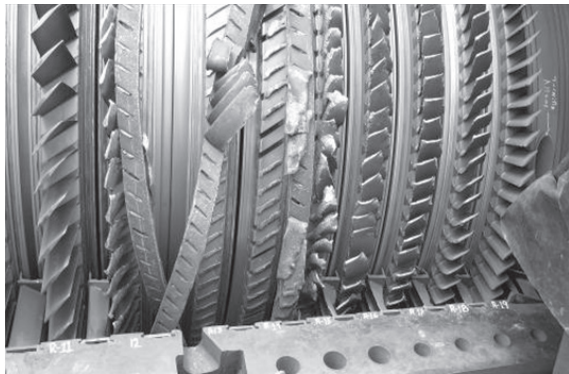
Fig. 10. Fracture surface of compressor diaphragm vane tenons, stage 13 with appearance of HCF
