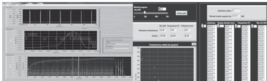
Fig. 11. Front panel of application for monitoring force versus time/displacement and panel for analysis of selected quantities, using signal filtration
