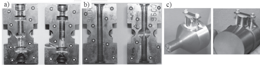
Fig. 8. Tools for forging carrying handles: a) dies for 2 nd operation, b) matrices for 3 rd operation, c) 2 nd and 3 rd operation punch with AE sensor
