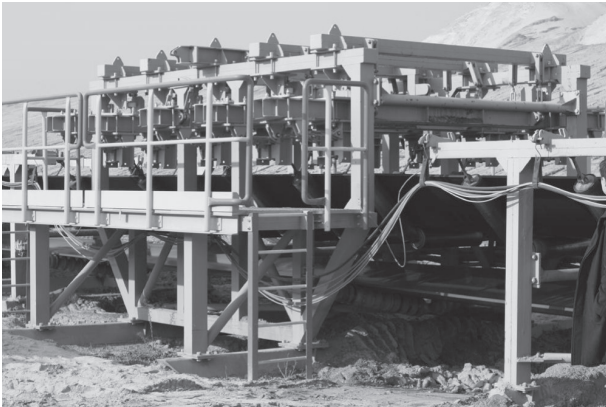
Fig. 14. Measuring segment for investigating motion resistance of single idler set
