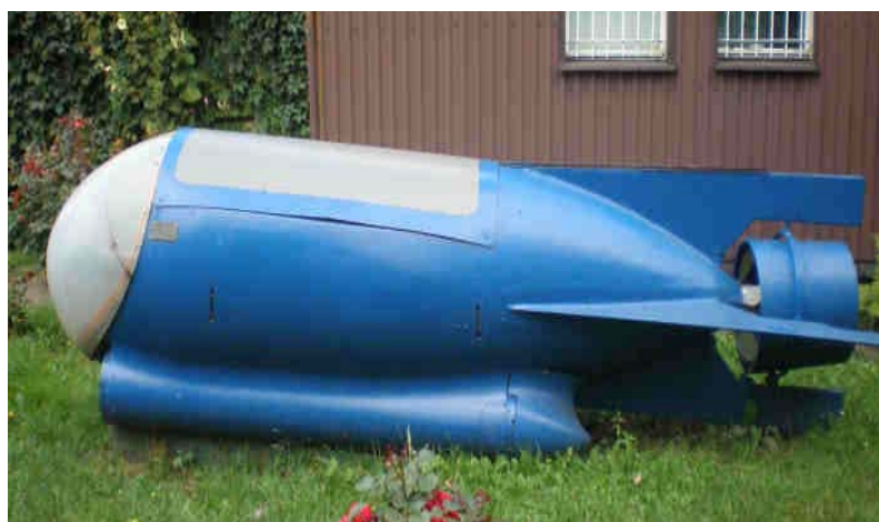
Fig. 18. The DPV Błotniak allowing a lying position (author's achieve).
