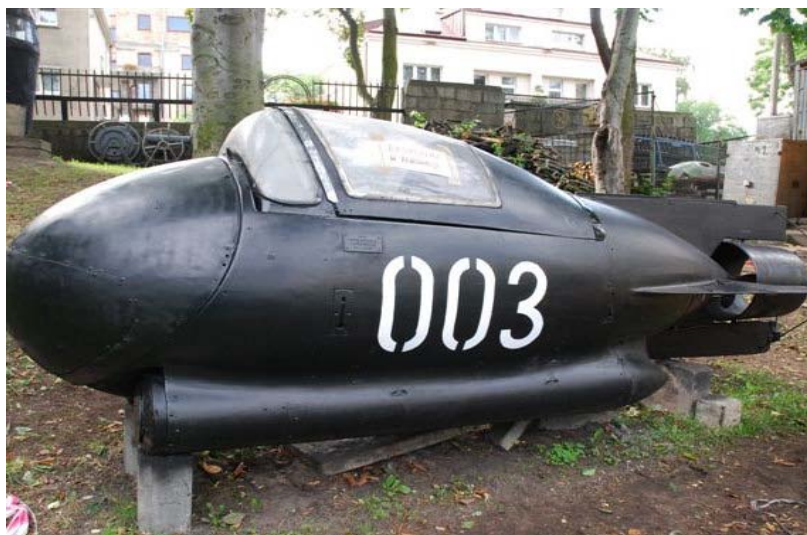
Fig. 17. The DPV Błotniak allowing a sitting position [27].
