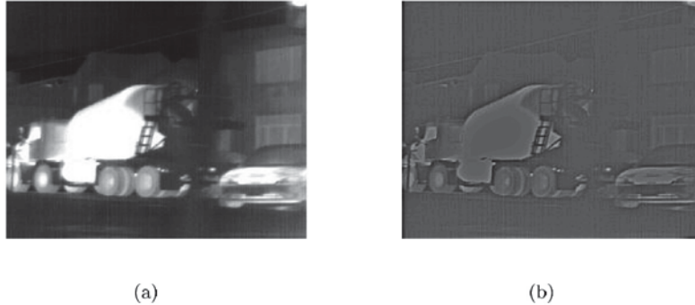
Figure 7: (a) Original thermal image, (b) Second order whitened image using Gluckman's orientation-averaged whitening procedure.
