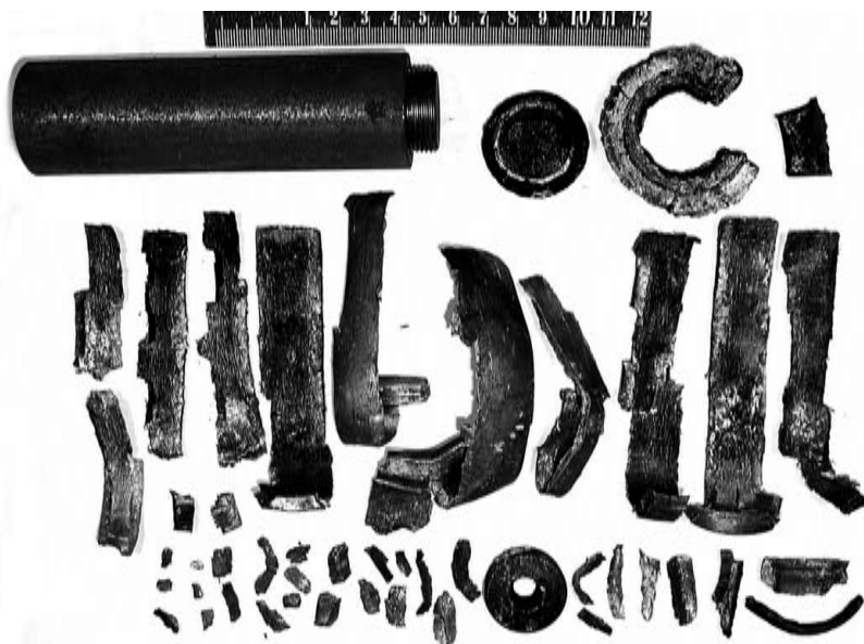
Figure 8. Photograph of steel confinement take and of its fragments after detonation of TATP.
