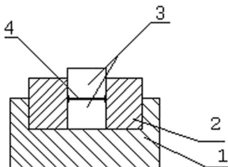
**Figure 1.** Experimental set: 1 – pallet; 2 –muff; 3 – rollers; 4 – sample.
