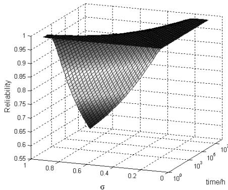
Fig. 9. The curved surface which depicts the reliability change with dispersion  $\sigma$  and time  $t$  simultaneously (Absolute change)
