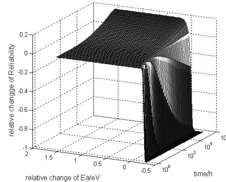
Fig. 8. The curved surface which depicts the reliability change with the activation energy  $E_a$  and time  $t$  simultaneously (Relative change)
