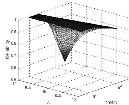
Fig. 5. The curved surface which depicts the reliability change with parameter A and time t simultaneously (Absolute change)
