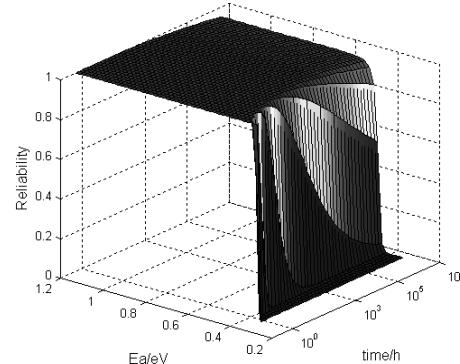
Fig. 7. The curved surface which depicts the reliability change with the activation energy  $E_a$  and time  $t$  simultaneously (Absolute change)
