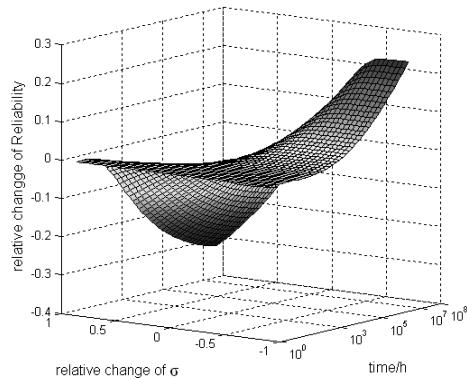
Fig. 10. The curved surface which depicts the reliability change with dispersion  $\sigma$  and time  $t$  simultaneously (Relative change)
