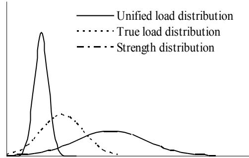
Fig. 1. Illustration of load unification and extended load-strength interference relationship
