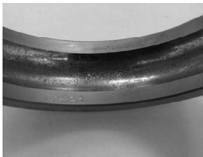
Fig. 6. Outer raceway spalling of P301C
