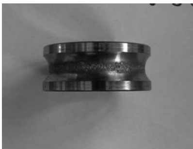
Fig. 7. Inner raceway flaking of P301D
