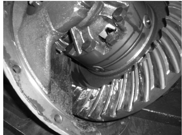
Fig.9. Fracture photo of rear axle gear
