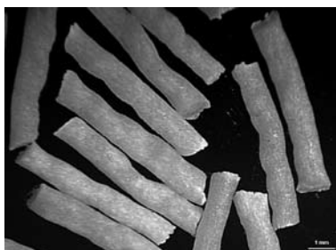
Figure 3. Examples of real shapes of analysed fine-grained tube propellant B.
