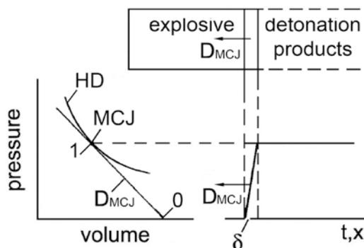
**Figure 1.** Michelson-Chapman-Jouguet detonation. Explosive transforms into detonation products simultaneously with its compression within the detonation wave shock front  $\delta$  (zero reaction zone model). HD: Hugoniot adiabat for detonation wave. 01: Michelson straight line.  $D_{MCJ}$ : MCJ detonation velocity.
