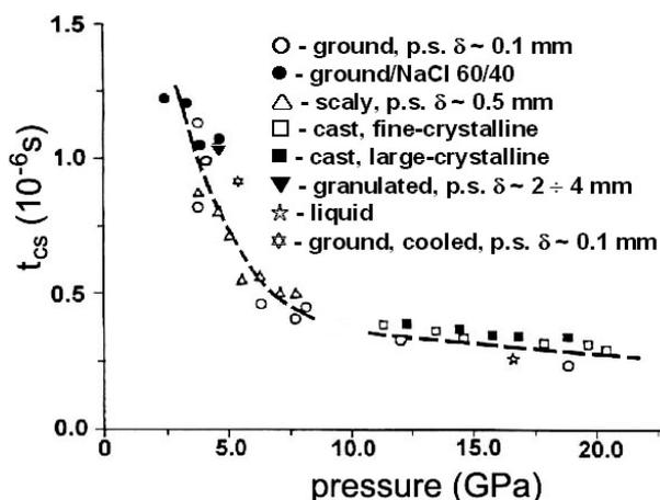
**Figure 3.** The dependence of chemical spike time  $t_{CS}$  on the pressure  $P$  of TNT charges detonation. p.s.  $\delta$ : explosive particle size  $\delta$ .
