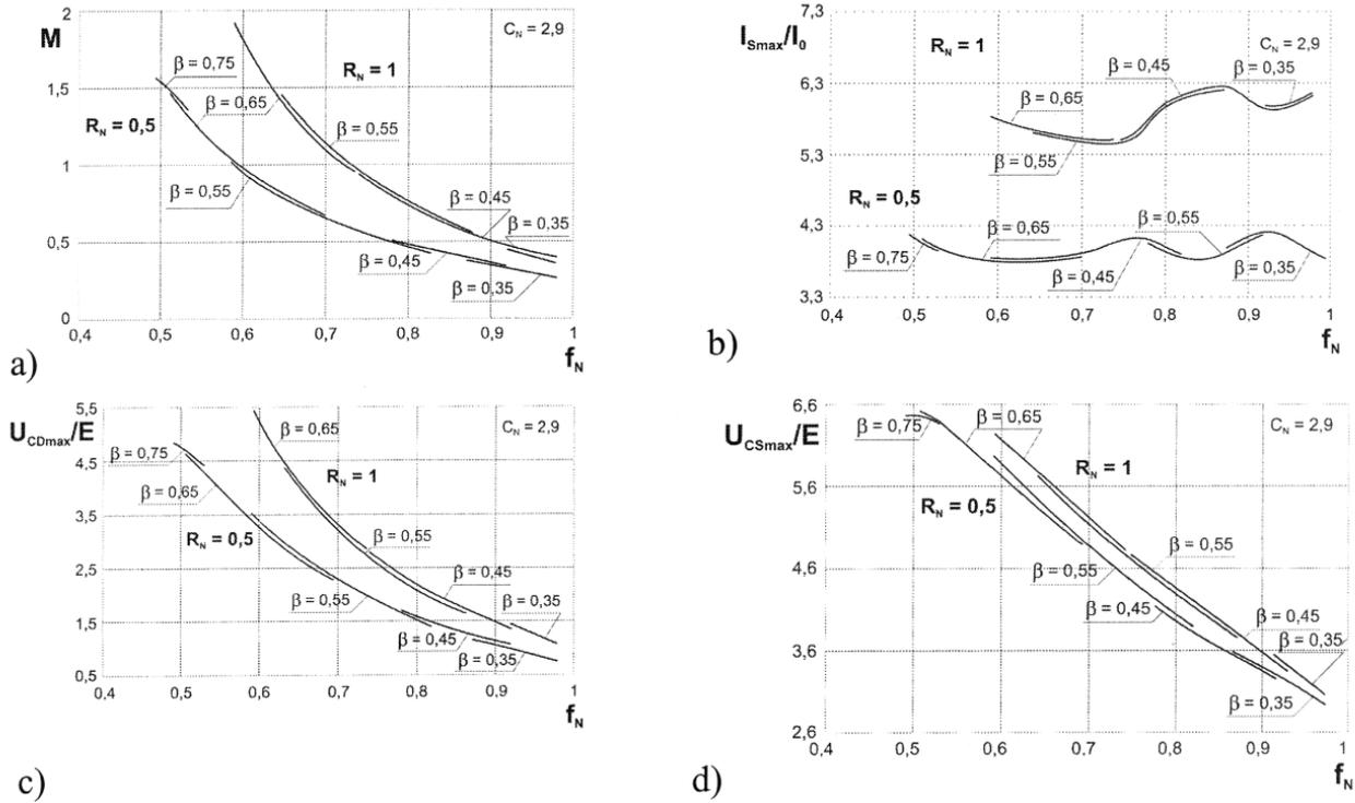
Fig. 7. Control characteristics for ZVS Cuk MRC in relative units,  $C_N = 2.9$ ,  $R_N = 0.5$ ,  $R_N = 1$ ; a) conversion ratio  $M$ ; b) maximum transistor current  $I_{Smax}/I_0$ ; c) maximum diode voltage  $U_{CDmax}/E$ ; d) maximum transistor voltage  $U_{CSmax}/E$
