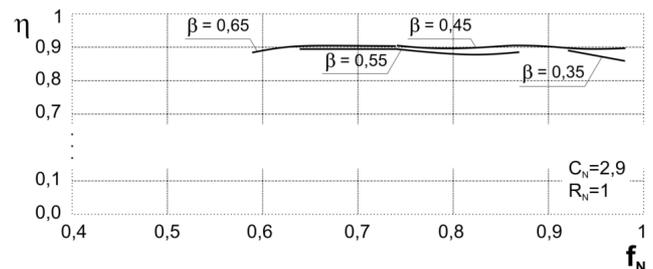
Fig. 10. Efficiency  $\eta$  of ZVS Cuk MRC,  $C_N = 2.9$ ; a)  $R_N = 0.5$ ; b)  $R_N = 1$
