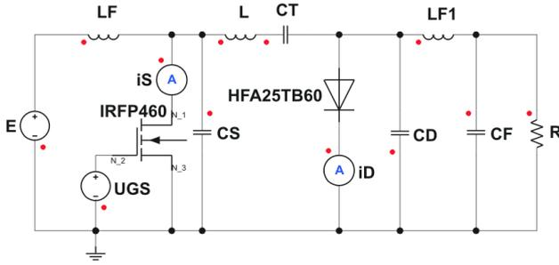
Fig. 4. Simulation model of ZVS Cuk MRC
