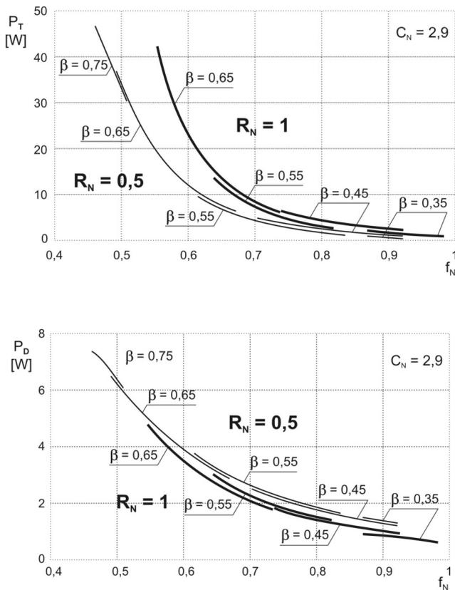
Fig. 8. a) Total transistor power losses  $P_T$ ; b) total diode  $D$  power losses  $P_D$
