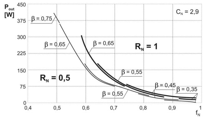
Fig. 9. Output power  $P_{out}$  of ZVS Cuk MRC
