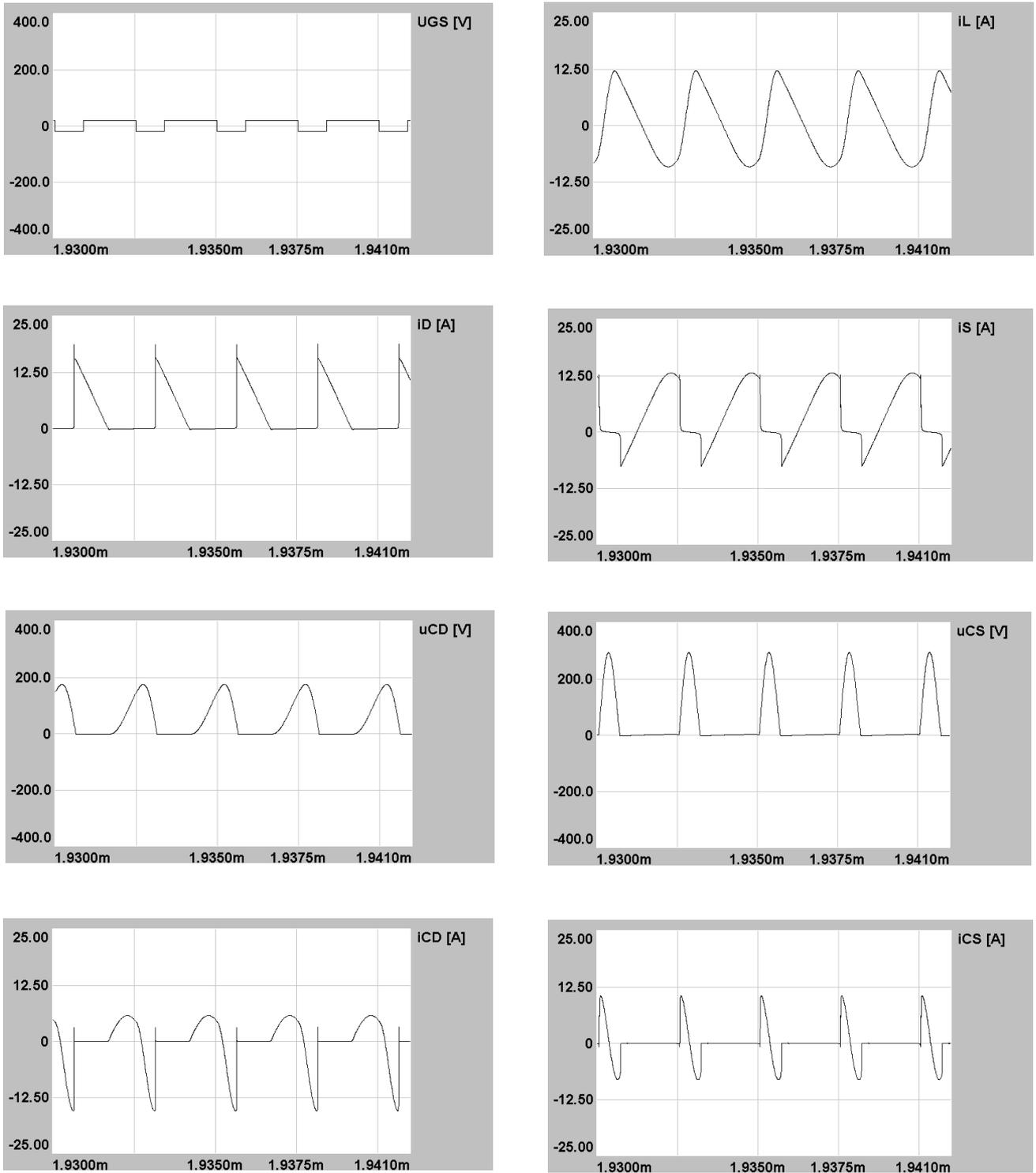
Fig. 6. Simulation current and voltage waveforms in ZVS Cuk MRC,  $C_N = 2.9$ ,  $R = 14.91\Omega$ ,  $U_O = 50.5V$ ,  $I_O = 3.4A$ ,  $f = 400kHz$  ( $f_N = 0.59$ ),  $\beta = 0.65$ ,  $\eta = 0.89$ ,  $P_{in} = 197W$ ,  $P_{out} = 175W$
