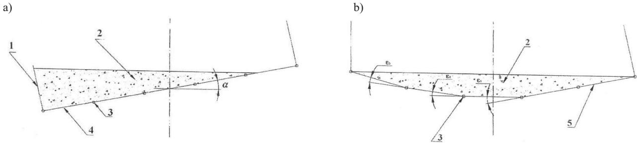
Fig. 1. Distribution of the screened material on the cylindrical sieve in the transverse inclination: a- sections of the cylindrical sieve arranged in a flat way (flat sieve model), b- extremely raised sections, 1- side passive surface, 2- cleaned material, 3- articulated joint of the section, 4- flat-arranged sections, 5- section of the cylindrical sieve,  $\alpha$  - inclination angle of the flat sieve,  $\epsilon_1, \epsilon_2, \epsilon_3$  - inclination angle of the cylindrical sieve section
