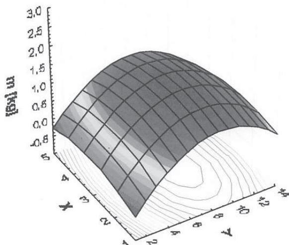
Fig. 8. Distribution of the grain mass  $m$  under the two-plane sieve at the main plane inclined at an angle  $\beta = -10^\circ$  „simulation of the uphill movement” for  $\alpha = 0^\circ$  and inclination angle of the half-open section  $\delta = 25^\circ$ , X1 - X5 – sections of the two-plane sieve, Y1-Y14 – measurement zones
