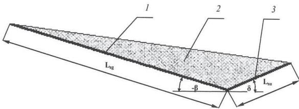
Fig. 3. Distribution of the screened material on the two-plane sieve inclined at  $\beta$ ; 1- main sieve plane, 2- grain mass to be cleaned, 3- adjustable half-open part of the sieve,  $L_{sg}$  - length of the main sieve plane,  $L_{su}$  - length of the half-open part of the sieve,  $\beta$ - inclination angle of the sieve basket (up the hill),  $\delta$ - angle of the additional sieve plane inclined from the horizontal plane.
