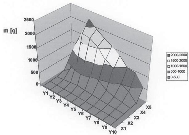
Fig. 6. Distribution of the grain mass  $m$  under the cylindrical sieve inclined at an angle  $\alpha = 10^\circ$  “simulation of the movement along the contours”, X1 – X5 sections of the cylindrical sieve, Y1 – Y10 measurement zones
