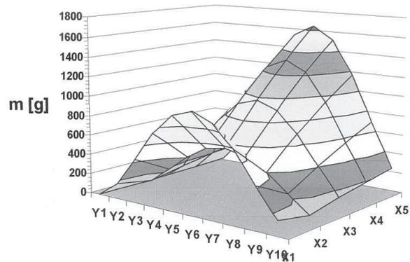
Fig. 7. Distribution of the grain mass  $m$  under the canopy sieve inclined at an angle  $\alpha = 10^\circ$ ; inclination angle of the section canopies  $\gamma = 10^\circ$ , X1 - X5 – sections of the canopy sieve, Y1-Y10 – measurement zones
