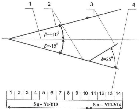
Fig. 5. Deflection scheme for the main and half-open planes of the two-plane sieve from the horizontal plane  $\beta$ ,  $\delta$ - deflection angle of the half-open plane; 1- horizontal plane, 2- main sieve of the separator, 3- half-open sieve of the separator, 4- measurement points,  $S_g$  - Y1 – Y10 – measurement zones under the main sieve,  $S_u$  - Y11 – Y14 - measurement zones under the half-open sieve
