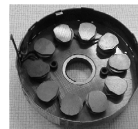
Fig. 20. Left side of stator
