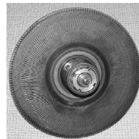
Fig. 17. Drawing of DC PM disc motor built-up plan
