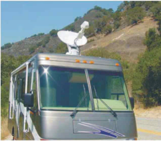
Fig. 4 Vehicle RV with satellite antenna (left side) and a map of satellite links (right side) [7]
