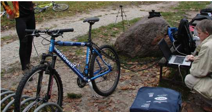
Fig. 3. Bicycle with the measurement sensors prepared for the test ride
