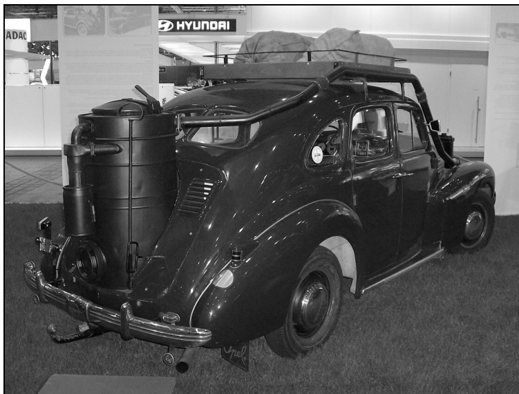
Rys. 4. Samochód Opel z generatorem w bagażniku Fig. 4. Opel vehicle with the wood gas generator in the luggage boot
