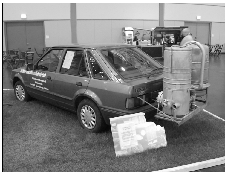
Rys. 4. Samochód Opel z generatorem w bagażniku Fig. 4. Opel vehicle with the wood gas generator in the luggage boot
