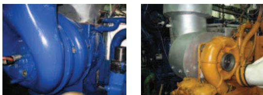
Fig. 1. PBS Turbo PDH-35 type axial-flow turbocharger on SULZER main engine type 8AL25/30 (left) and NAPIER C-045/C radial-flow turbocharger on SULZER auxiliary engine type 6AL20/24 (right)
