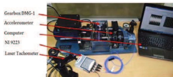
Fig. 1. Experimental gearbox and measuring system
