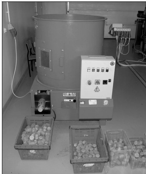
Fig. 1. Hydraulic briquetting machine with an open chamber from POR, model: JUNIOR
