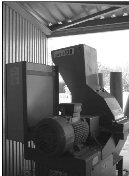
Fig. 2. Beater mill for biomass grinding from POR, model: KING c120
