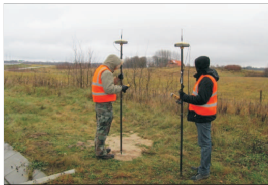
Fig. 3. Survey of points by means of the RTK method
