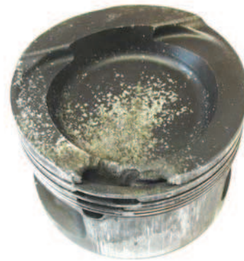
Fig. 6. A piston damaged (burnt out) by an incorrect modification of the engine's control software
