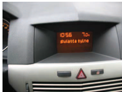
Fig. 3. Diagnostic message informing the user about rear lamp circuit failure
