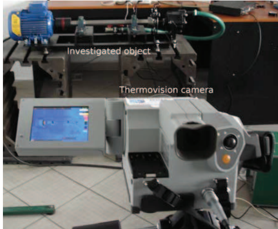
Fig. 2. Investigated object and applied infrared camera
