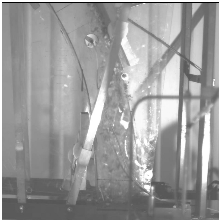
Fig. 2. Motion of chaff particles in the first spout section
