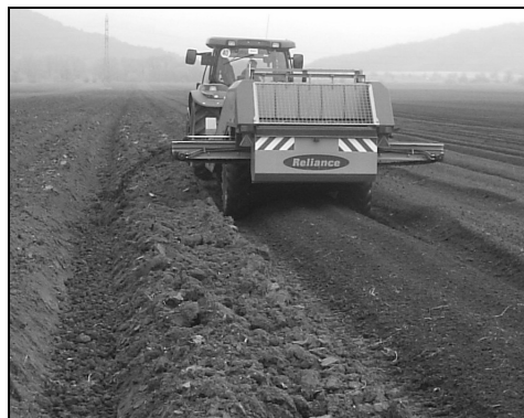
Fig. 5. Stone separator for potato cultivation soil preparation
