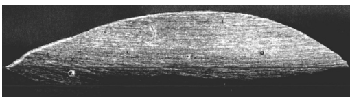
Fig. 4. Surfacing profile of the FIDUR 10/60 material
