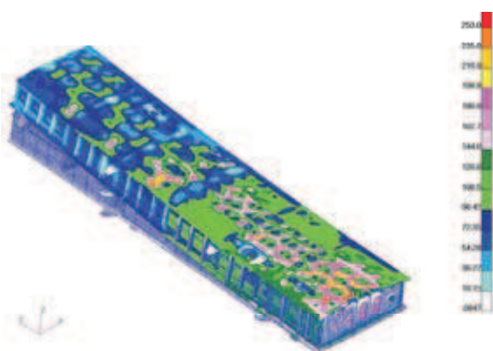
Fig. 5. Reduced stress (by H-M-H11) [MPa] and the displacement in the model wing. The apparent local loss of stability
