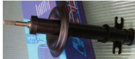
Fig. 3. The twin tube hydraulic shock absorber for front suspension of Fiat Punto
