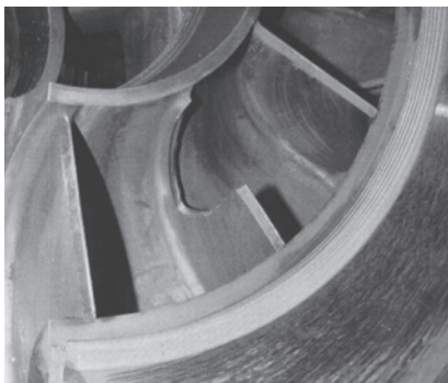
Fig. 1. View of the damaged diaphragm vane
