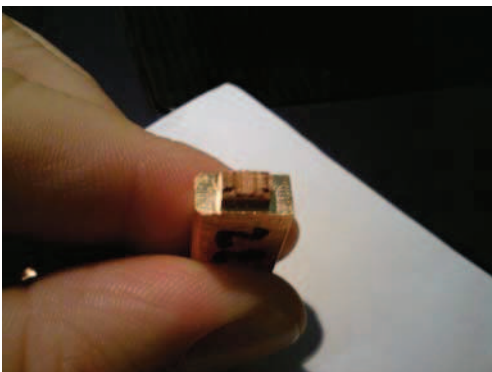
Fig. 4. View of the fracture of a beam with a P-type notch
