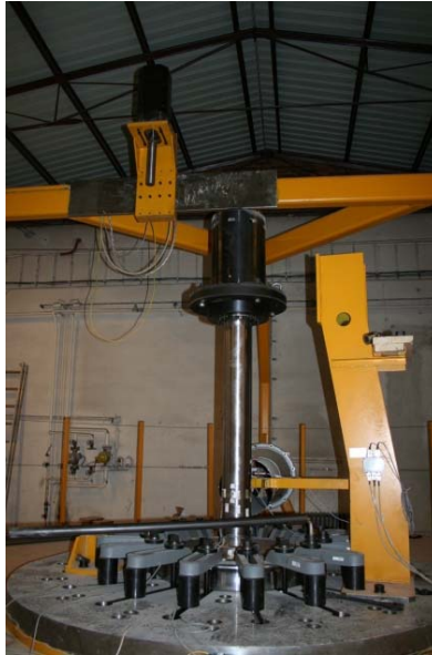
Fig. 4. Resonance testing equipment dedicated to fatigue testing of railway axles
