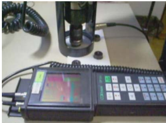
Fig. 12. View of a peel-testing device used for the measurement of adhesion of applied layers
