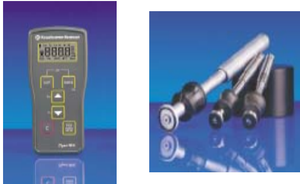
Fig. 8. Dynamic ball hammer used in BONATRANS GROUP, including a view of a probe used for measurement of hardness by reflection method
