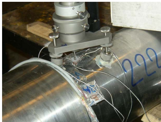
Fig. 9. View of the drilling device used for destructive measurement of residual stresses
