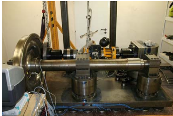
Fig. 3. A view of a wheel after shot-peening and of the testing equipment built in BONATRANS GROUP a.s. dedicated to railway wheels testing
