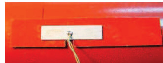
Fig. 5. Piezoelectric sensor for collecting strains
