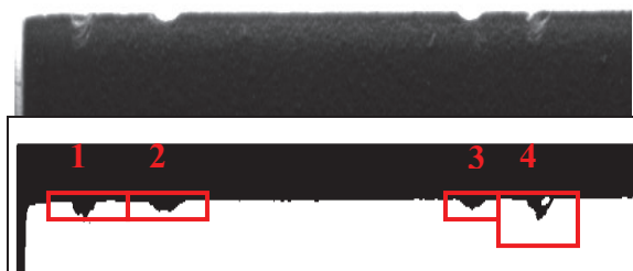
Fig. 8. Exemplary results for tile with damaged edge.
