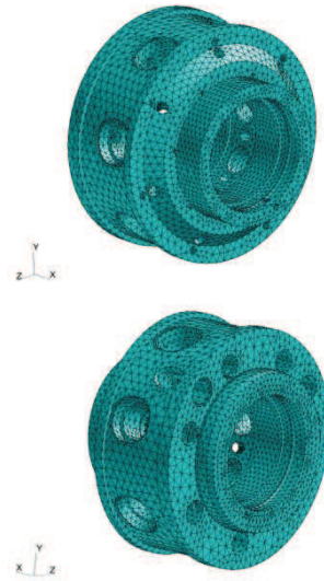
Fig. 10. The finite elements model of the body of pump
