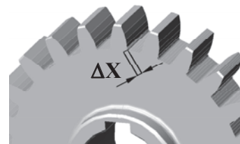
Fig. 1. The modelled wheel defect in the form of a crack in the tooth root
